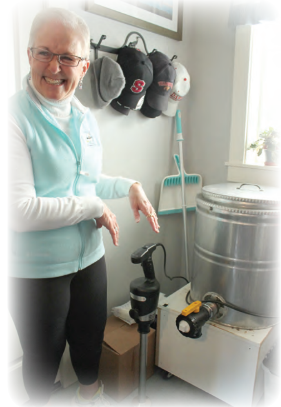
Lyn Faas of Bunny's Bath uses a custom-made jacketed boiler and industrial-sized immersion blender to process her liquid soap products. Photos by Kathie Meyer
